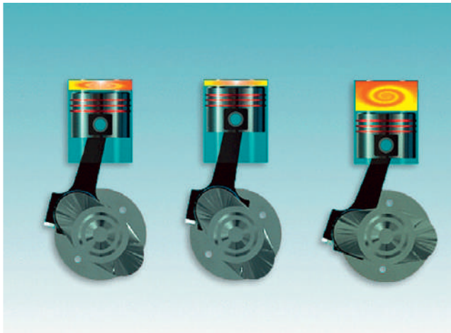
Figure 2.23 Ideal, retarded and advanced ignition point
